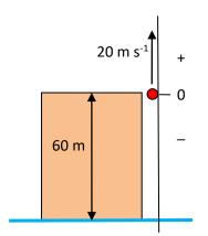
We want to find the time when the ball hits the sea. According to our conventions this happens when the position of the ball is -60 m. Then we go to a formula involving displacement and time i.e.
