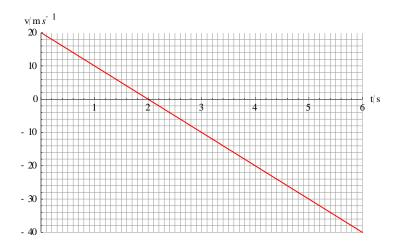
What is the gradient of this graph? What is the area under the graph from t = 0 to t = 2 s and what does it represent?
